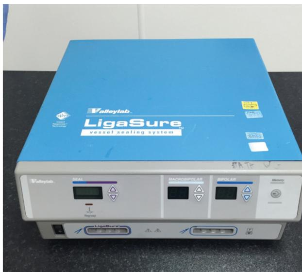
**Figure 1:** The dedicated generator for use with Ligasure vessel sealing handpieces. This model has been superseded but is affordable and still available on the reconditioned market
